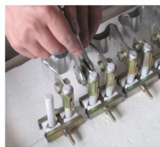
Step 2: Unscrew the fixture of the top end of the heating element carefully
