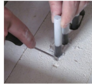
Step 6: Lift the MoSi2 rod around 10mm. The top end of U rod should have 10 mm distance to furnace bottom to avoid heater heat expansion distortion.
