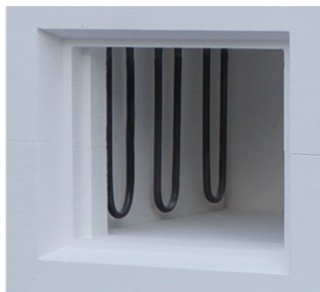
Step 7: Keep 10mm distance from U rod top to furnace bottom as picture .
