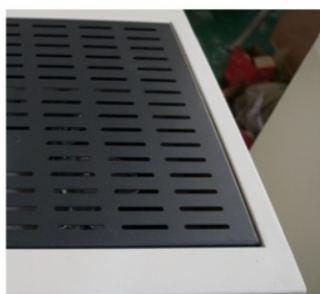
Step 1: Take off the furnace top cover
