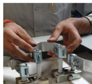
Step 3: Remove the Connecting Alumina Foil Clamp
