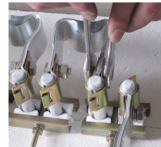
Step 9: Reassembly the Connecting Alumina Foil Clamp
